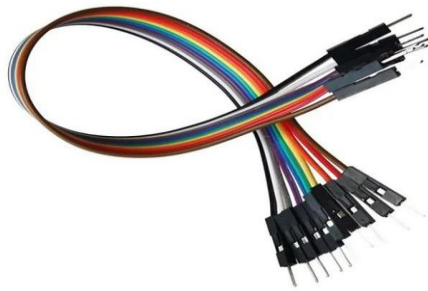
Fig. 15: Jumper Wires for Circuit Interconnection
