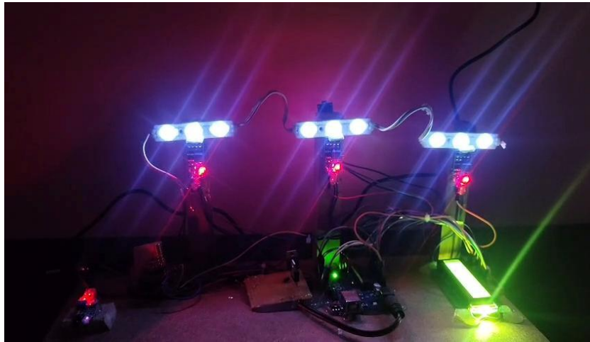
Fig. 20: Result – Street Lights at Full Brightness (100%) When Vehicle Detected
