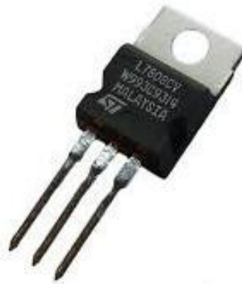
Fig. 13: 7805 Positive Voltage Regulator (LM78XX Series)
