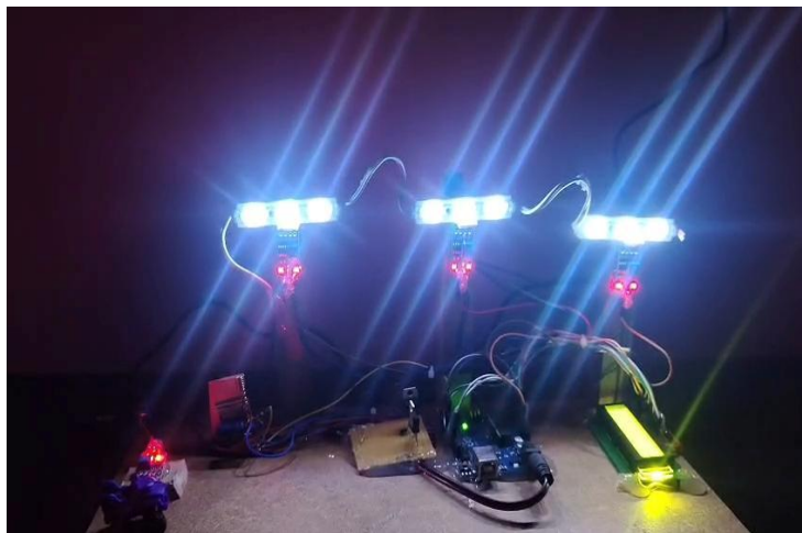
Fig. 21: LCD Displaying Light Failure Alert – "LIGHT 1 FAILED PLEASE CHECK"
