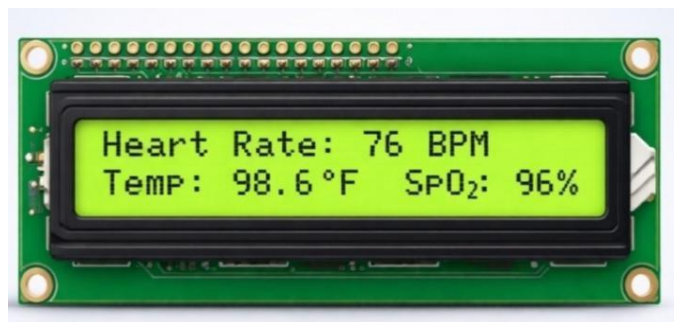
Fig. 6 — 16×2 LCD Displaying Real-Time Heart Rate, Temperature and SpO 2
